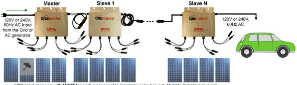
4 DC Input channels with MPPT for each solar panel to maximize solar harvest. Multiple CyboInverters can daisy-chain making installation truly "plug-and-play."
