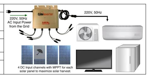
Product: CyboInverter - 4 Channel 1.25KW AC Assisted Off-Grid Solar Inverter CIM-1200Sa Standalone Off-Grid Model for 220V, 50Hz AC Loads.
