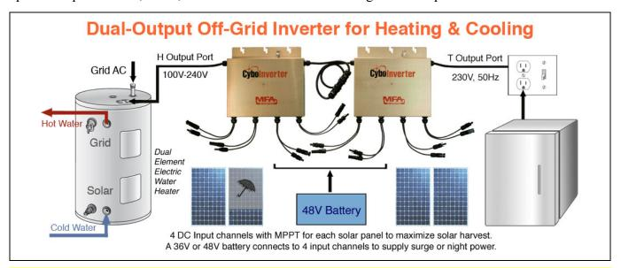
Product: 2.5KW Dual-Output Off-Grid CyboInverter Twin Pack for Microgrids CIM-1200H/T1, H/T2 H Port: 100V-240V, T Output Port: 230V, 50Hz
