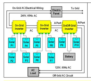
When the grid is on, the inverter works like a regular on-grid inverter that meets UL1741 and IEEE1547 standards having over / under voltage shutdown; over / under frequency shutdown; and anti-islanding.
